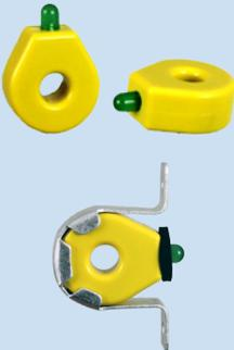
Used to monitor the status of the power supply to heater elements, motors, contactors or fans. If the load fails the LED does not illuminate, indicating a fault in the circuit. The LED body can be panel mounted or free standing.
